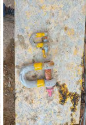
Lifting Tools and tackles color coding system
